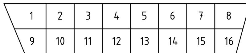
Figure 4 — Contact designation for vehicle connector mating end view
